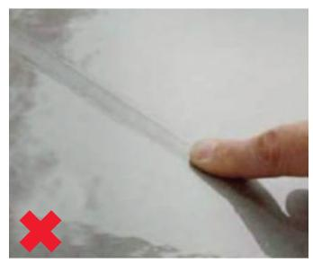
For an optimum result of the surface finish, it is essential that the demoulding oil layer is homogeneous and as thin as possible:
